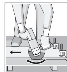
The power tool must always work in an up-grinding motion. Otherwise there is a risk that it will be pushed uncontrollably out of the cut. For best results when cutting profiles and rectangular tubing, start at the smallest cross section.
