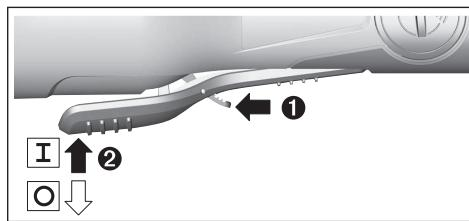
To **start** the power tool, push the unlocking lever (9) forwards and then push the on/off switch (8) up.
