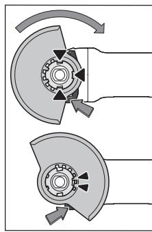
Place the protective guard **(10)** onto the holder on the power tool until the coding cams of the protective guard are aligned with the holder. When doing so, press and hold the unlocking lever **(1)**. Press the protective guard **(10)** onto the spindle collar until the shoulder of the protective guard is sitting on the flange of the power tool and rotate the protective guard until it audibly clicks into place.
